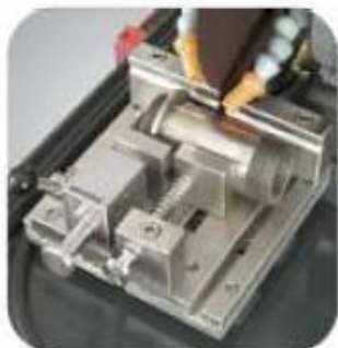
Stainless steel clamping devices and T-slotted table
